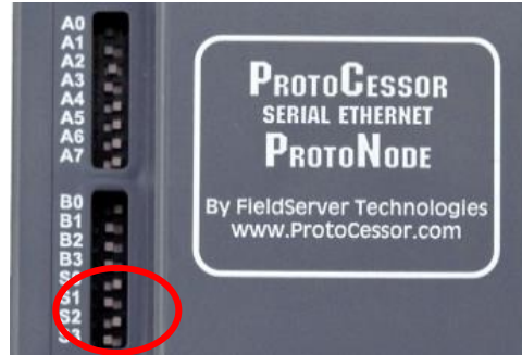
S Bank DIP Switch Location
