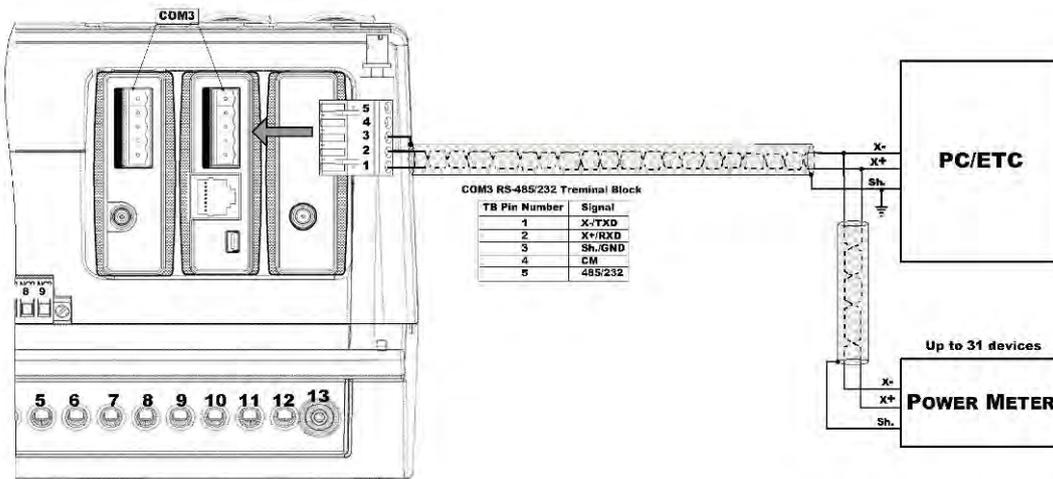
Figure 17: Serial Communication Network Connection - RS-485 COM3
