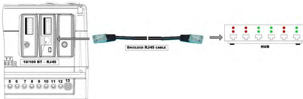
**Figure 19: 10/100BT Ethernet RJ45 Connection**
