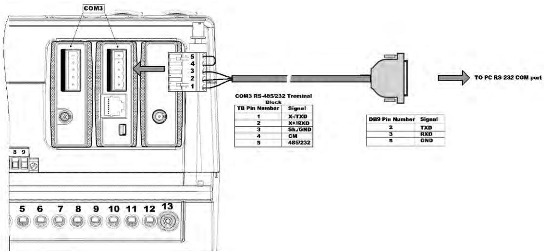
Figure 18: Serial Communication Connection - RS-232 COM3
