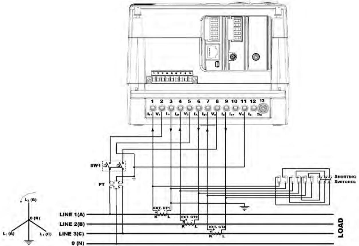
Figure 10: Three Wire Wye Connection Using 2 PTs, 3 CTs - Wiring Setup: 3LL3 or 3Ln3
