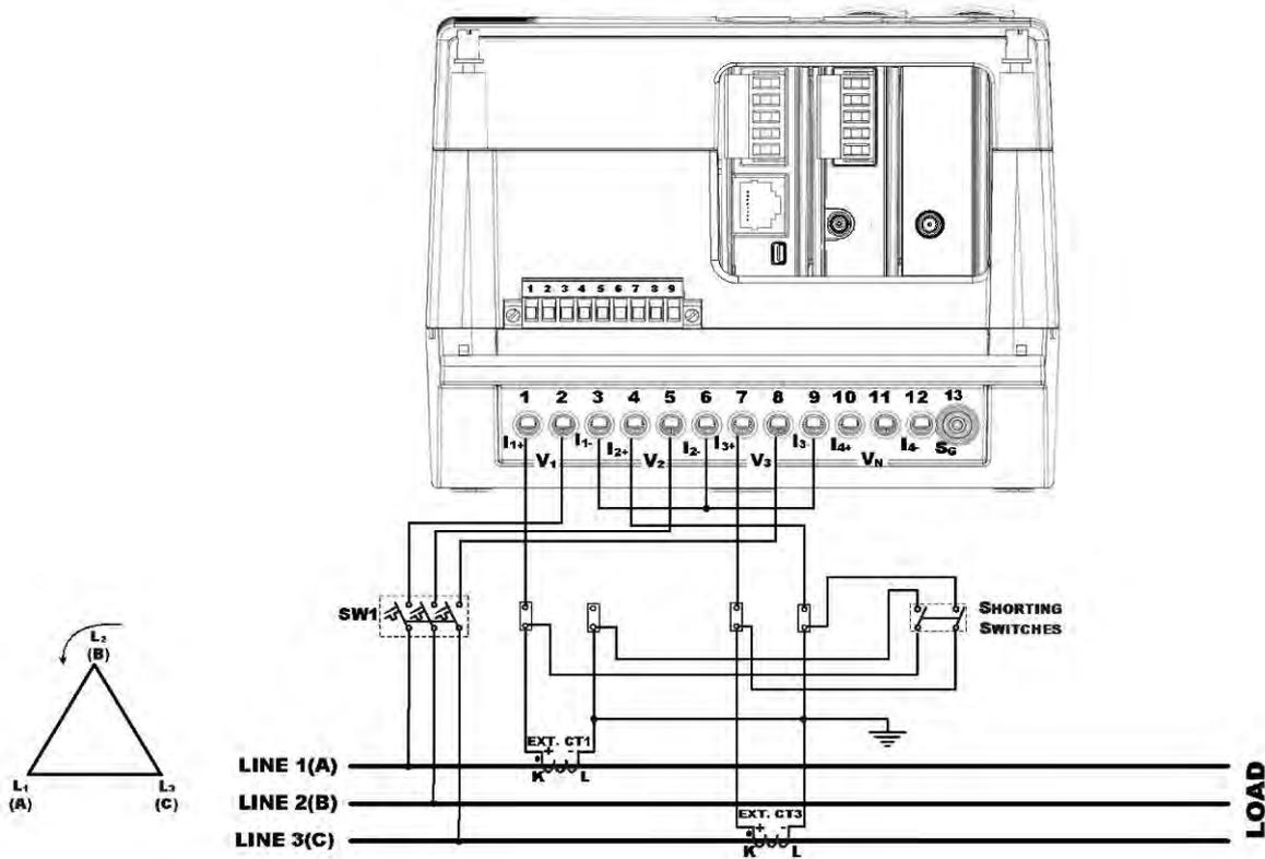
**Figure 6: Three Wire Using 2 CTs - Wiring Setup: 3dir2**
