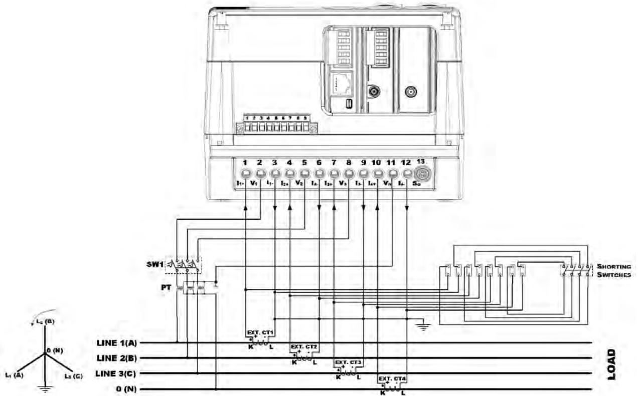
Figure 8: Four Wire WYE Connection Using 3 PTs, 3 (4) CTs - Wiring Setup: 4LL3 or 4Ln3
