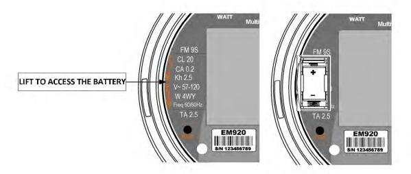
Figure 35: Memory Backup - Lithium Battery Replacement
