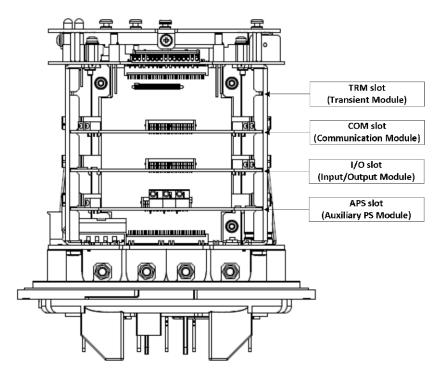
Figure 4: EM920 internal structure
