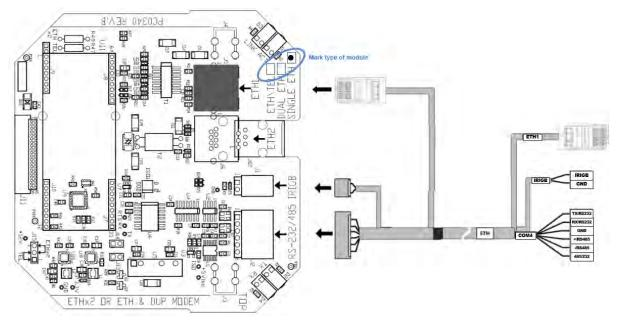
Figure 25-b: Single ETHERNET module (new)
