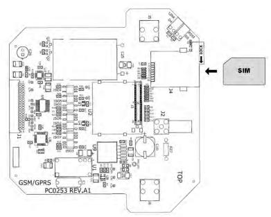
Figure 24: GSM/GPRS module - SIM card assembly
