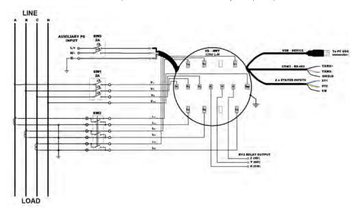
Figure 6: FORM 9 Typical Electrical Installation
