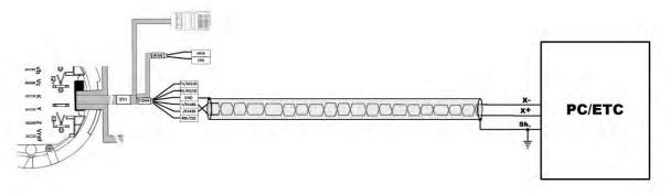
Figure 28: Serial Communication Network Connection - RS-485 COM4
