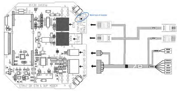
Figure 25-c: Double ETHERNET module
