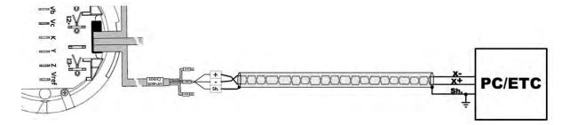
Figure 22: Serial Communication Network Connection - RS-485 COM3
