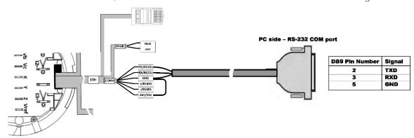
Figure 29: Serial Communication Connection - RS-232 COM4
