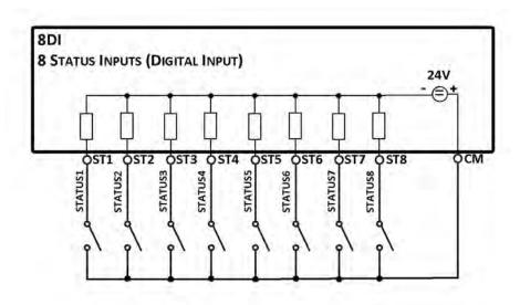
Figure 17: 8DI module STATUS Input Connection
