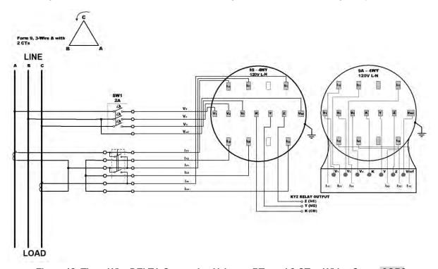
Figure 12: Three Wire DELTA Connection Using no PTs and 2 CTs - Wiring Setup: 3OP2
