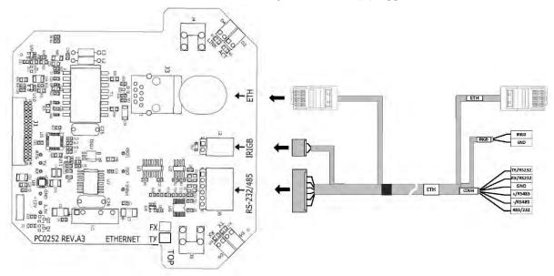
Figure 25-a: Single ETHERNET module (old)
