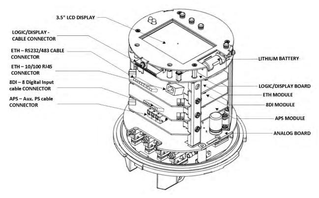
Figure 3: EM920 internal structure
