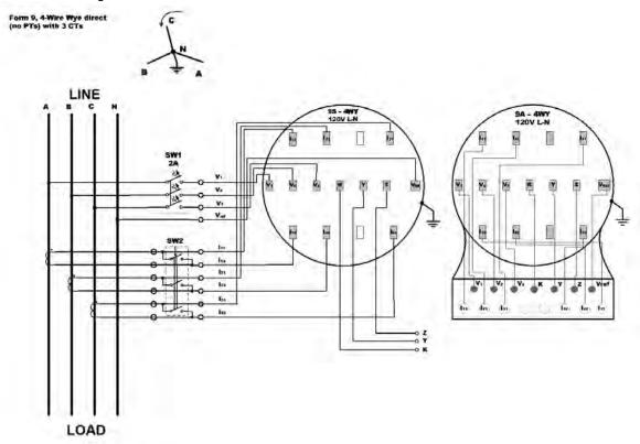
Figure 8: Four Wire WYE Connection No PTs Using 3CTs - Wiring Setup: 4Ln3
