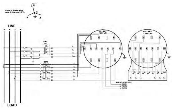
Figure 9:Four Wire WYE Connection Using 3 PTs and 3(4) CTs - Wiring Setup: 4Ln3
