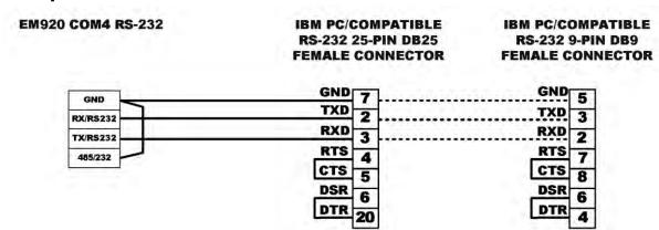
Figure 33: RS-232 Simple 3-wire Connection , 25-pin or 9-pin PC COM Port
