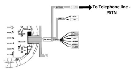
Figure 31: MODEM connection
