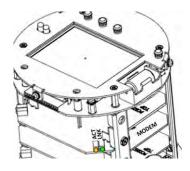
The **MODEM** module provides additionally to COM4 indication GREEN LEDS, MODEM indication leds:
