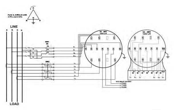
Figure 11: Four Wire DELTA Connection Using 3 PTs and 3 CTs - Wiring Setup: 4LL3
