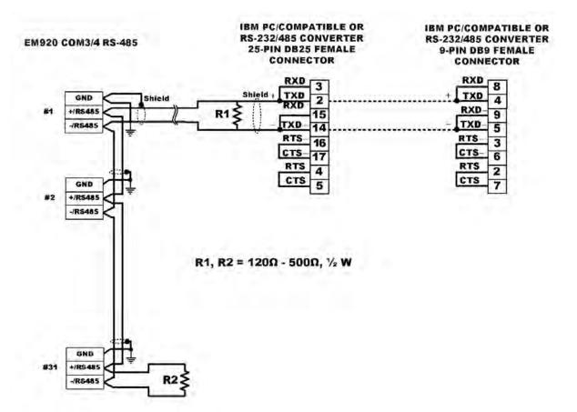
Figure 34: RS-485 Multidrop Connection, 25-pin or 9-pin PC COM Port
