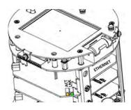
The *ETH* module provides additionally to COM4 indication GREEN LEDS, ETHERNET indication leds:
