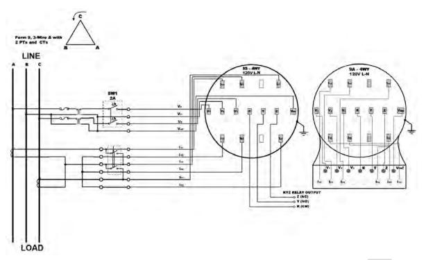
Figure 13: Three Wire DELTA Connection Using 2 PTs and 2 CTs - Wiring Setup: 30P2
