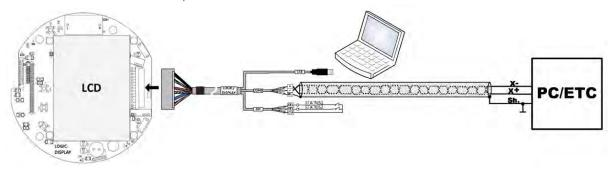
Figure 14:LOGIC/DISPLAY Cable
