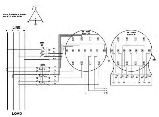
Figure 10: Four Wire DELTA Connection Using no PTs and 3(4) CTs - Wiring Setup: 4LL3
