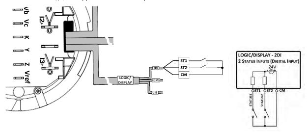
Figure 15: 2DI LOGIC/DISPLAY STATUS Input Connection
