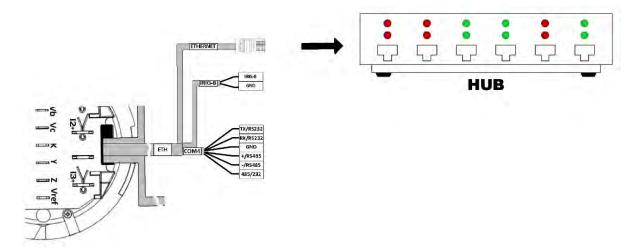
Figure 30: ETHERNET connection
