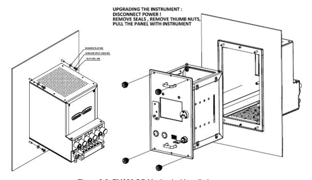
Figure 2-3: EM920-DP Mechanical installation
