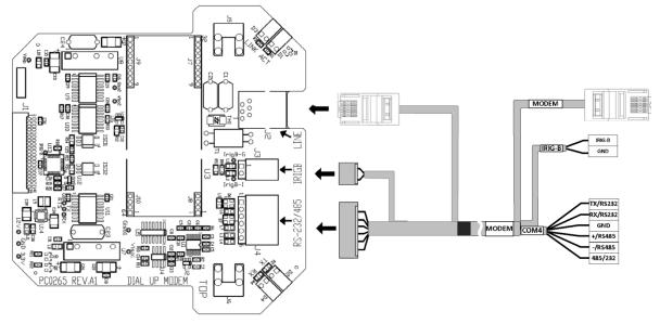
Figure 26-a: MODEM module (old)
