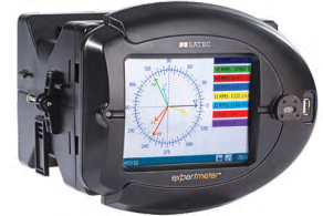
PHASOR MEASUREMENT UNIT
