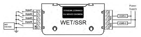
Figure 2-25 4DI/2RO WET Contact/SSR
