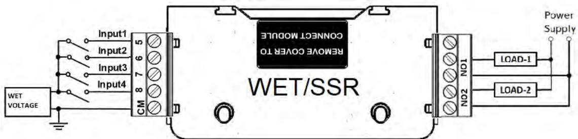
Figure 2-25 4DI/2RO WET Contact/SSR
