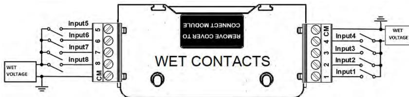
Figure 2-22 8 DI - Digital Input Connection – Wet contact model
