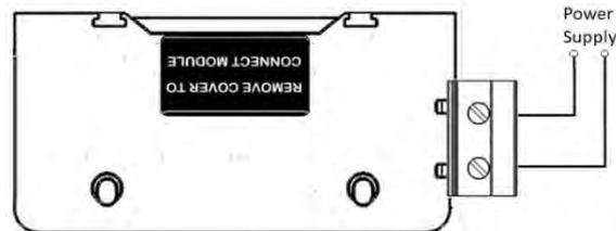
Figure 2-26: AUX\_PS Module Connection
