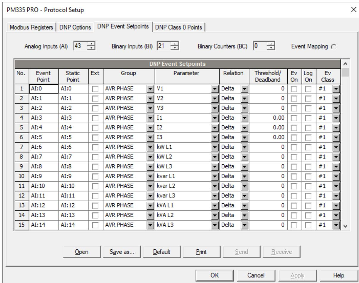
3. For AI and BC points, select a relation and an operating threshold or a deadband to be used for detecting events. All thresholds are specified in primary units. The following relations are available:
