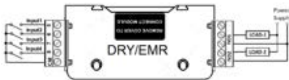
Figure 2-13 Dry Contact Inputs Connection
