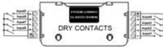
Figure 2-10 8DI Dry Contact Module Connection
