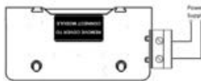
Figure 2-9 Auxiliary Power Supply Connection
