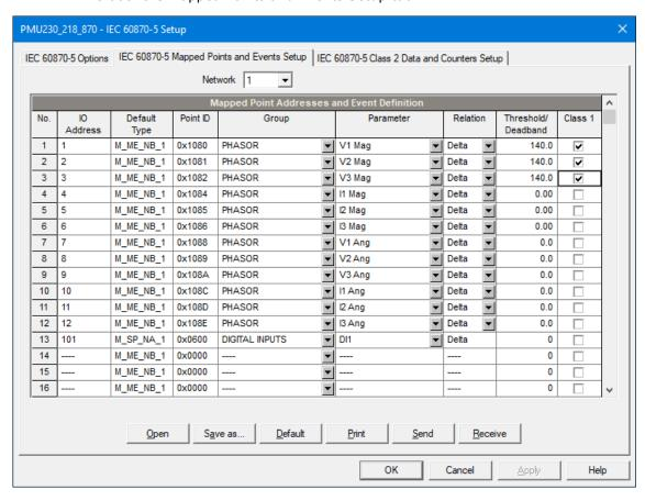
2. Select an object group and parameter for the points you want to remap. Object types and addresses are assigned automatically based on the initial mapped address and the default static type you selected for the object type in the IEC 60870-5 Options Setup (See Section 6.1).
