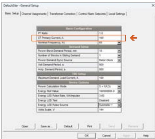
When configuring the meter, make sure to set the value of the HACS CT's primary current, either via the front panel of the unit or via the PAS software.
