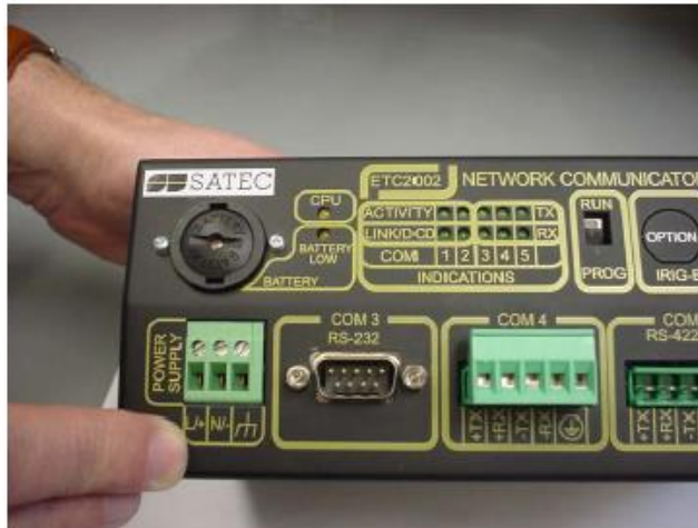
Figure 7-1 Battery Housing Location of the Panel
