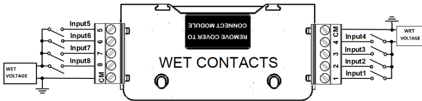
Figure 2-22 8 DI - Digital Input Connection – Wet contact model
