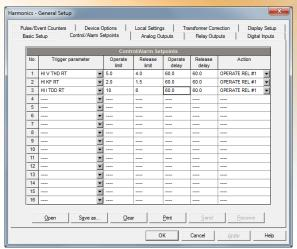
**Figure 5: Harmonics Setpoint Example**
