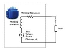
**Figure 1: Simple Electrical Network**
