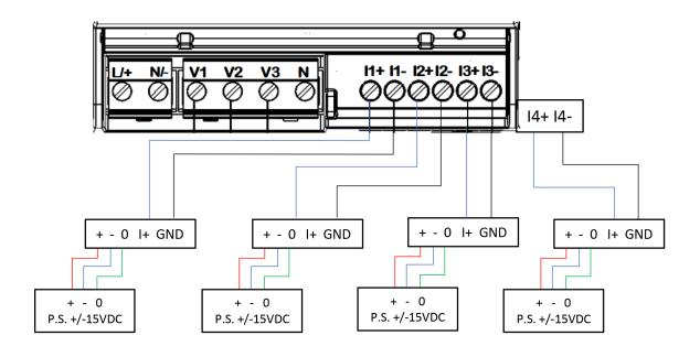
It is mandatory to setup the PRO meter to DC mode using PAS Software.
