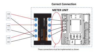
For DC High Voltage connection: recommended distance between SATEC VRM and SATEC meter should not exceed 2 meters, using cables featuring minimum 600V insulation.
